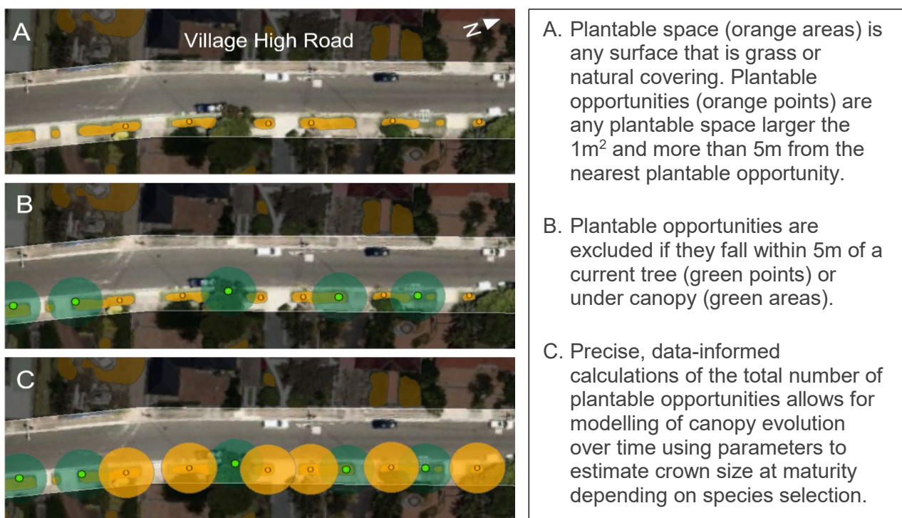
Figure F1. Example from a section of Village High Road, Vacluse, of how the STP tool identifies plantable opportunities.
