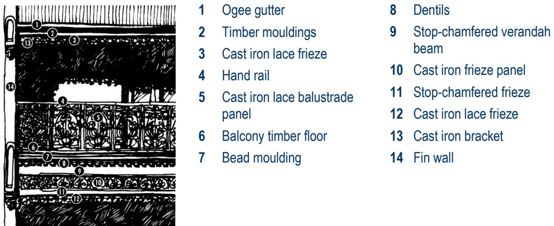
FIGURE 17 Typical Victorian terrace verandah elements
