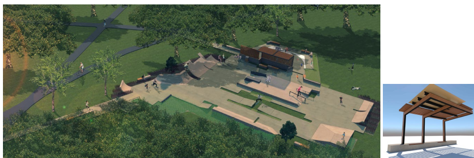
Figure 7.5 Aerial photo montage of the proposed Youth Facility and detail of the shade shelter that will separate the skate park from the basketball practice area. (Source: Concept 03 —Perspective 1, Convic 2018)
