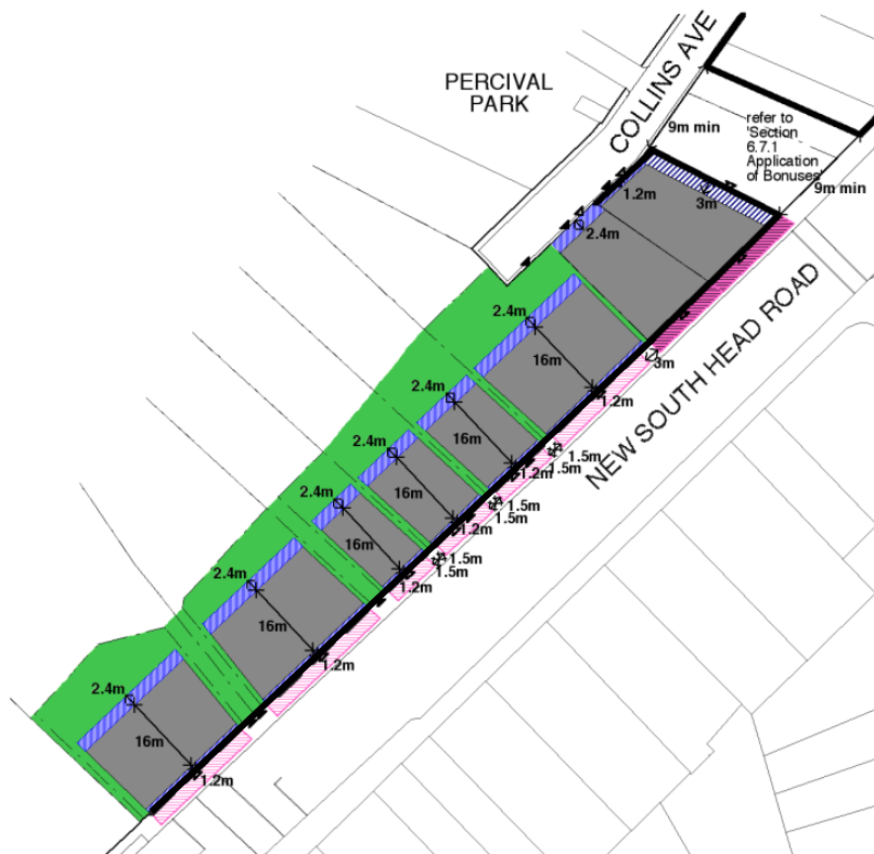
Ground floor level controls
