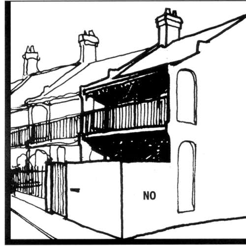
FIGURE 25 Boundary masonry fence
